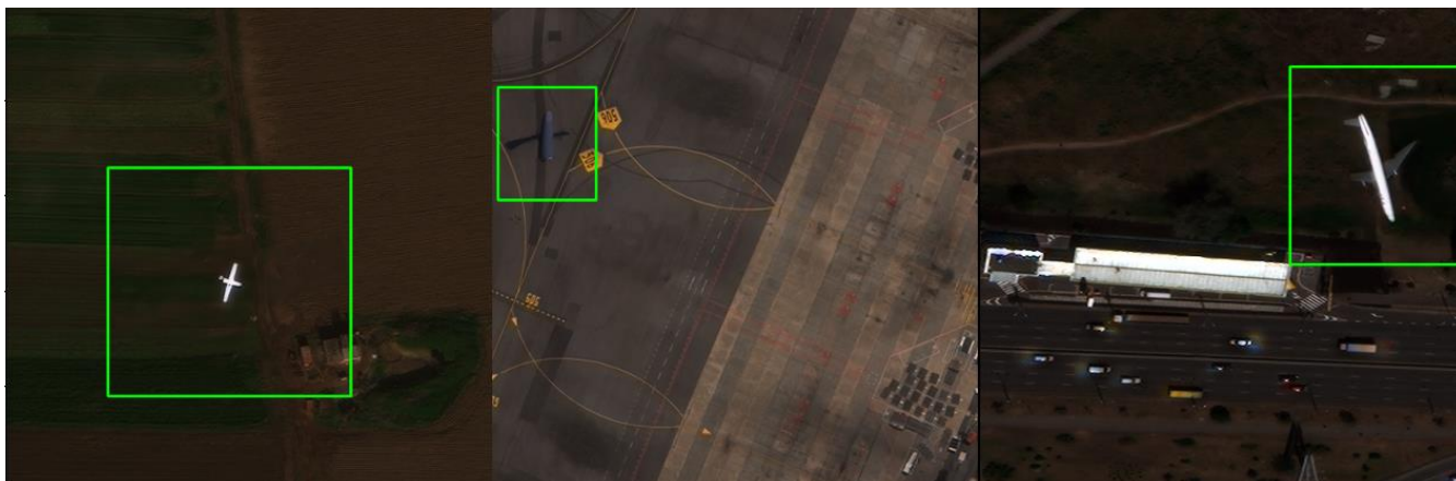
Figure 19 : Failure case with our unconditional model. Left : The plane generated doesn't fill the InPainting mask, thus the bounding box isn't adapted (solved with guidance). Middle: No plane is generated (solved with guidance). Right; some parts of the generated plane are missing. This last failure case occurs when we generate the plane in a 'random context' : an image with a background totally out of the distribution of the diffusion model's training dataset. With these images we usually chose a non squared inpainting mask to limit the amount of context the model would need to infer. These tighter masks cause in certain instances these failures to generate the whole plane.
